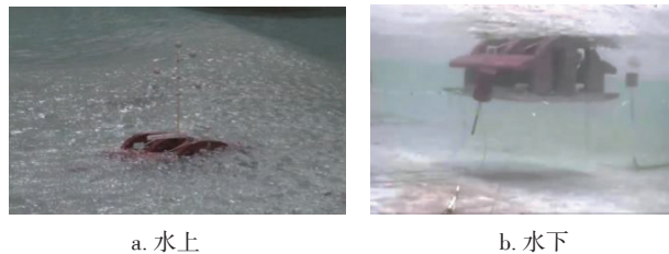
图 8 极限海况下鹰式装置与系泊系统动态响应 Fig. 8 Dynamic response of mooring system in extreme condition
