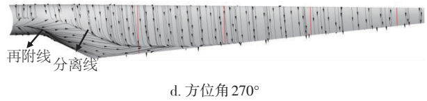
图 11 偏航 30°压力、流线与叶片表面极限流线分布 Fig. 11 Pressure, streamline and limiting streamline distribution on surface at different azimuth angle under yaw angle of 30°
