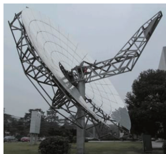
图1 25 kW 碟式聚光装置 (半径 6.65 m, 焦距 7.25 m) Fig. 1 25 kW solar dish concentrated device (radius is 6.65 m, focal length is 7.25 m)
